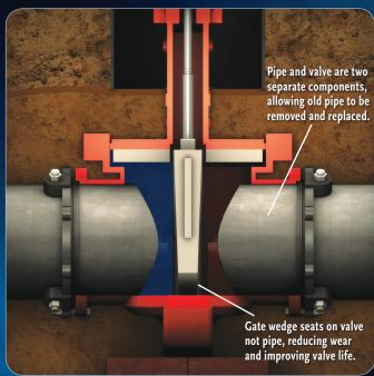
T eam's patented InsertValve™ delivers value, reliability and performance second to none. Unique valve characteristics include:
